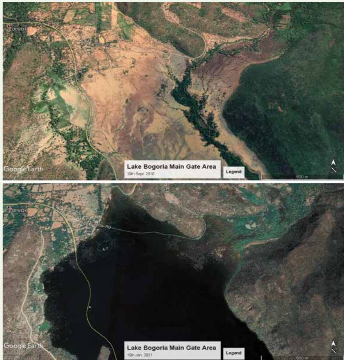
Figure 15: Google Earth image extract showing the status of the Northern end of Lake Bogoria on 10th Sept. 2010 compared to the status on 15th January 2021 clearly showing the location of the submerged roads and the position of the relocated road
